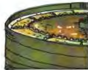
Clarifiers are used to clean steel plant water by letting solids settle out.
