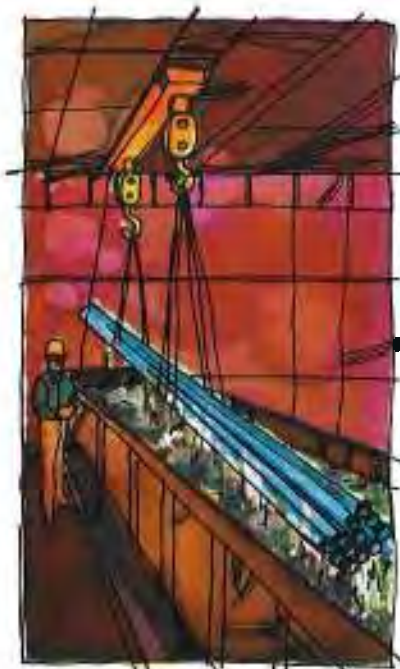
PICKLING (CLEANING) TUBES
