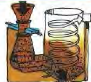
Venturi scrubbers spray water into dust-laden gases. Recovered solid particles may often be recycled.
