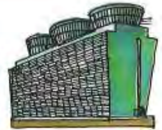
Cooling towers reduce temperature of cooling water so it can be used again and again.
